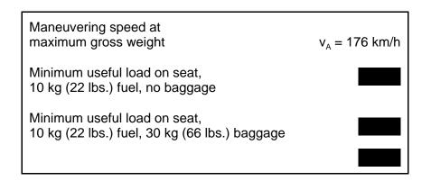
The following placard is attached to the instrument panel. The airspeed may be specified in a different unit, depending on the airspeed indicator.
