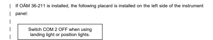
The following placard is attached to the left side of the instrument panel:
