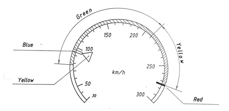
Green arc: 78 km/h - 210 km/h (42 kt - 113 kt) Yellow arc: 210 km/h - 275 km/h (113 kt - 148 kt) Red radial line at 275 km/h (148 kt) Blue radial line and yellow triangle at 95 km/h (51 kt) The following Placards must be attached/exchanged:
