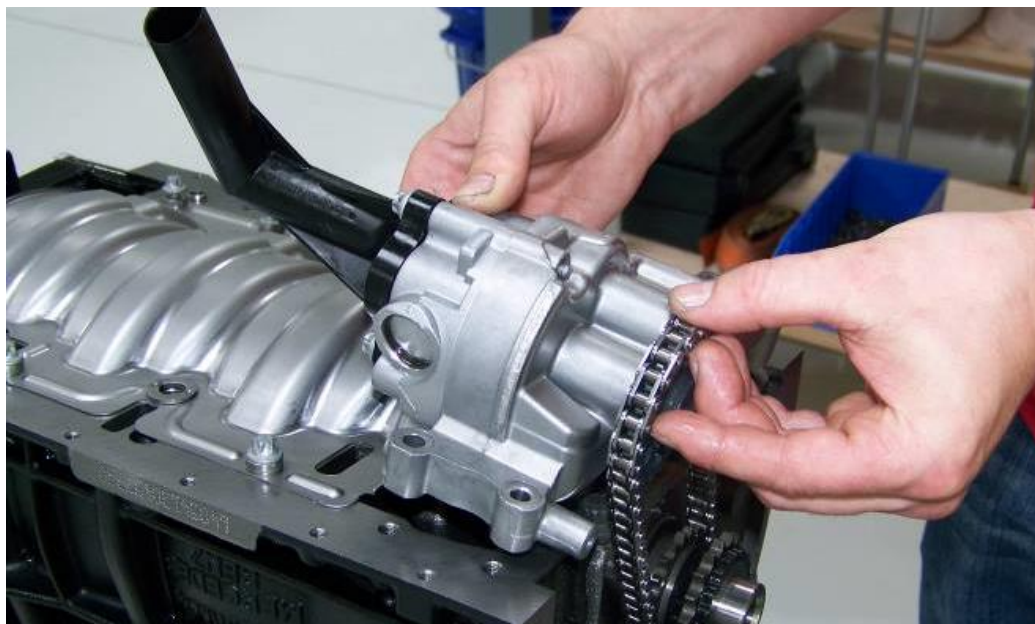
Fig. 14 Oil pump chain installation
