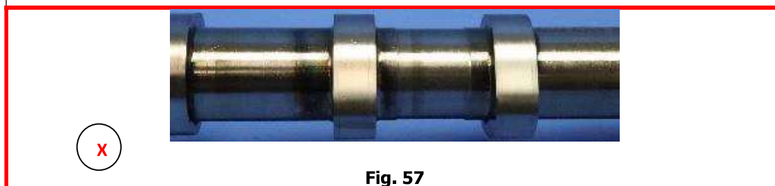
Examples of camshaft in not acceptable conditions
