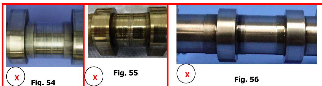
Examples of camshaft in not acceptable conditions
