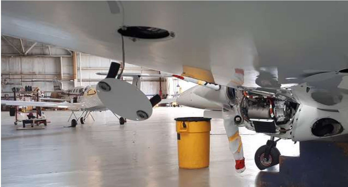
Figure 1. Vented access panel on the bottom of the wing.
