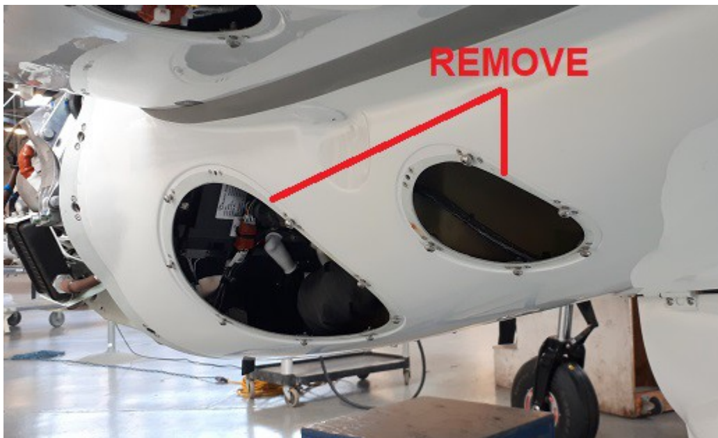
Figure 1. Access panels to remove.
