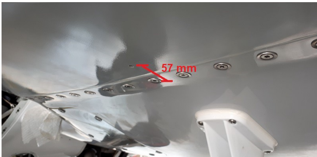
Figure 2. Drain hole in front of the landing lights.
