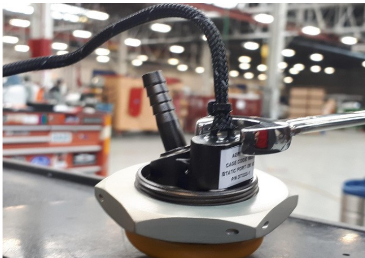
Figure 4. Hold the static port at the location shown when tightening the M40 nut.
