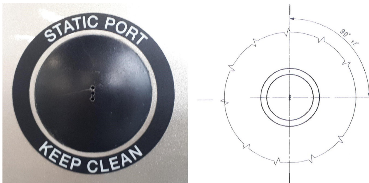
Figure 3. Left: static port from exterior. Right: orientation of the holes must be \pm 2^\circ from vertical.
