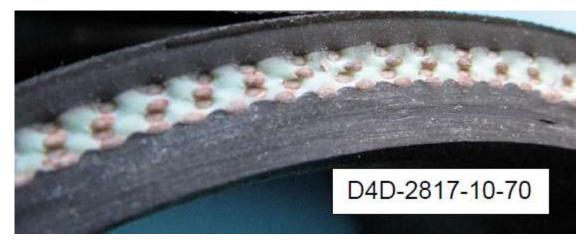
D4D-2817-10-70\_01, this fuel tank connection hose has an all black cross section and is not affected.
