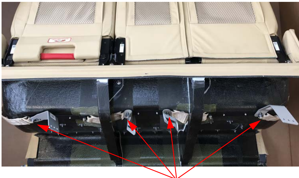
Bolt positions to inspect Figure1 - Middle Seat
