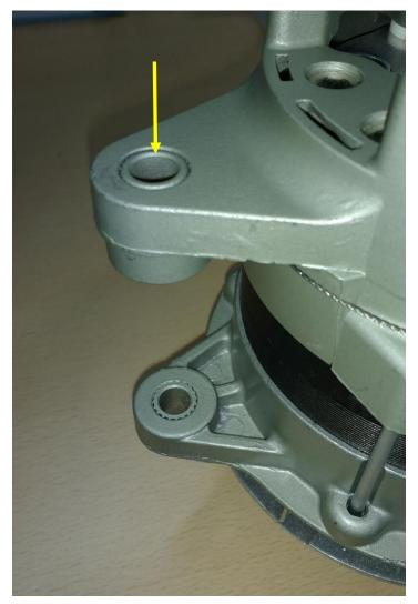
Ream the alternator housing with a 15H7 reamer.
