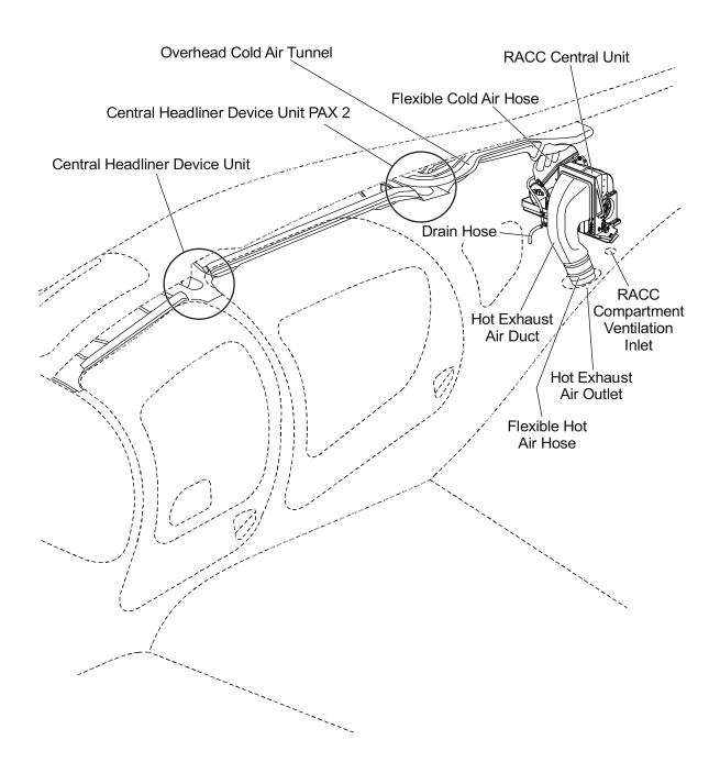
Figure 201 : RACC Central Unit Installation (if OÄM 62-005 is installed)
