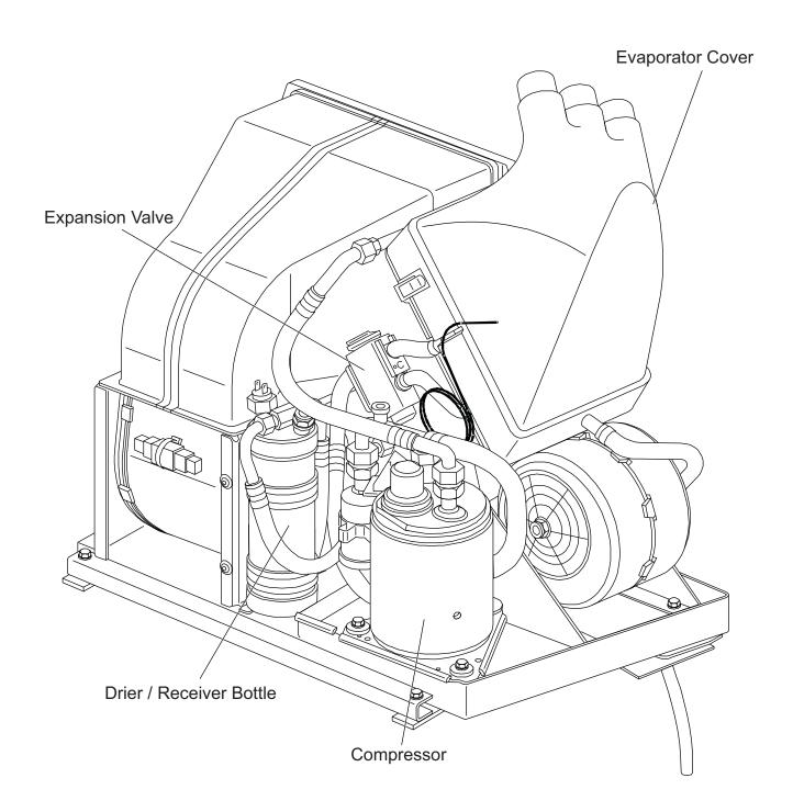
Figure 203 : Central Unit Back and RH Side (if OÄM 62-005 is installed)
