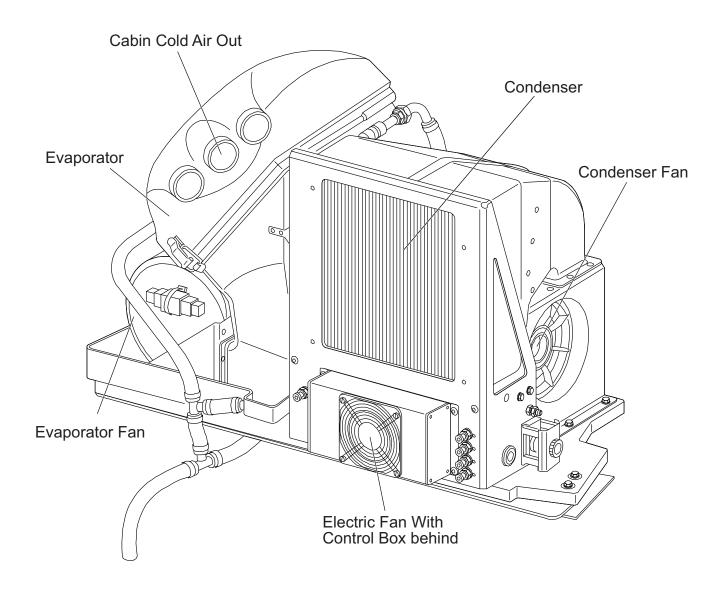
Figure 202 : Central Unit - Front and LH Side (if OÄM 62-005 is installed)
