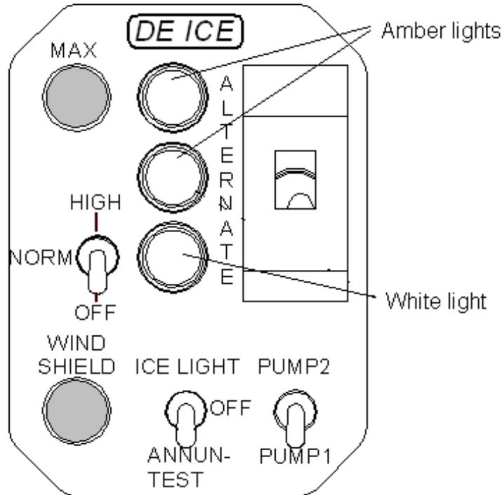
The OFF/NORM/HIGH switch operates the selected main pump and thus activates the system. It has 3 positions:
