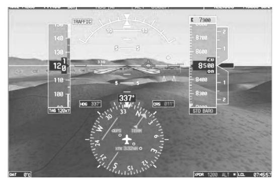
SVT provides additional features on the G1000 primary flight display (PFD) which displays the following information:
