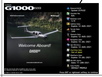
This 'System' number is the System Software Version. It correlates to the G1000 NXi, DA50 System Loader Card. For example:
