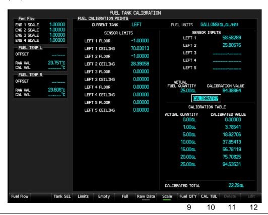
79 Select the left fuel tank, manually set ACTUAL FUEL QUANTITY to 0.00GL and select CALIBRATE? using the ENT key. Verify data entry and confirm the "Overwrite data" message by selecting YES and pressing the ENT key.
