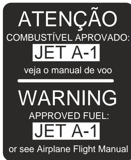
Figure 1 - Next to Each of the Two Filler Necks
