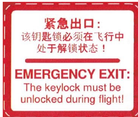
Figure 1 - Beside the Door Locking Device installed in the Passenger's Door
