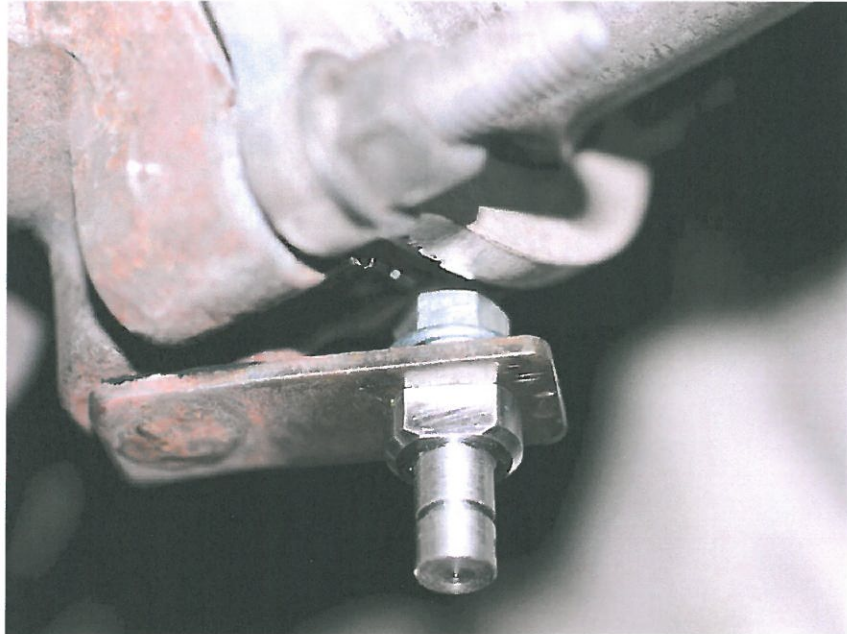
Fig. 6 Attachment of the new pin
