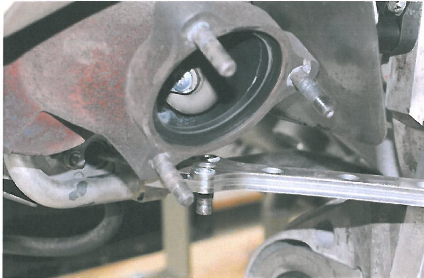
Fig. 2 Hold the waste gate lever steady
