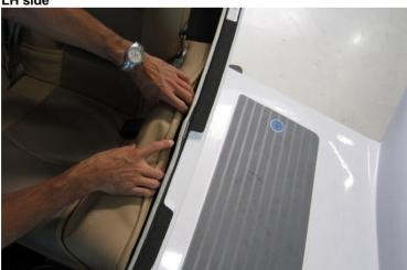
If LH side of passenger seat is completely lifted over lower edge of passenger entry, move passenger seat out through passenger entry. (two people are recommended for this work)
