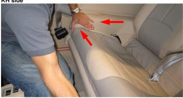
5 WHILE lifting LH side of passenger seat over lower edge of passenger entry.
