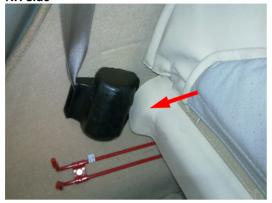
Slightly press RH side of passenger seat against fuselage and forward to create enough clearance on LH side.
