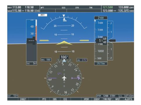
3. Upon successful completion of the pre-flight test, an aural alert will sound and the 'PFT' annunciation will clear. Continue to Step 5.9.2.
