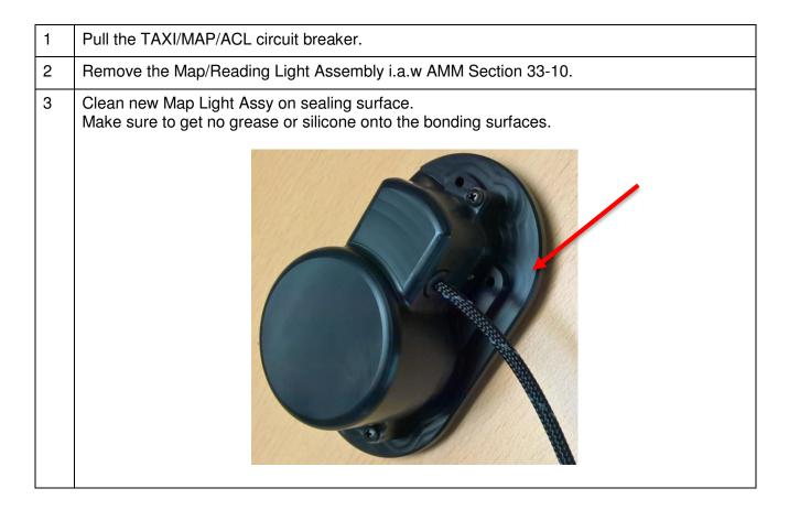
Remove the protective foil from the seal before installation on the new Map Light. Install the Map Light Seal on the Map Light.
