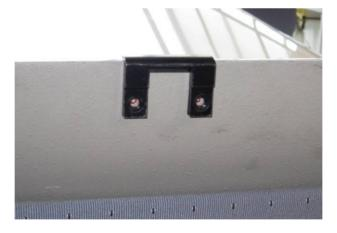
Remove the Retaining Bracket and drill the two holes with a diameter of 7mm (9/32 inch) and a depth of 7mm (9/32 inch) on the marked positions.
