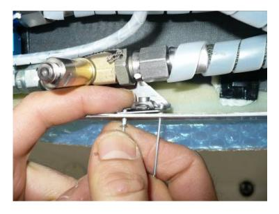
Check the correct valve position before mounting. Install the solenoid including the plug on the valve and secure it with the screw in a vertical position.
