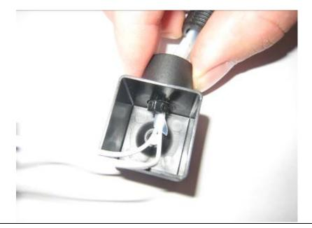
16 Assemble the plug and install it on the solenoid.
