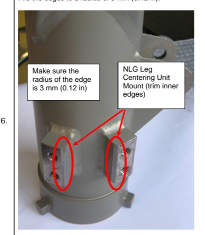
CAUTION: Make sure not to damage the NLG surface while filing the edges.
