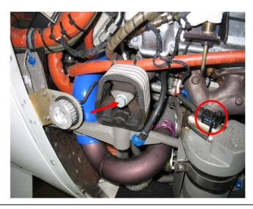
Remove the four bolts which fix the engine support bracket to the cylinder head and remove the engine support bracket.
