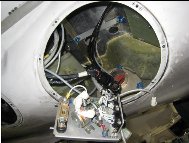
ECU-compartment with partially disconnected relay box and removed TAE-harness.
