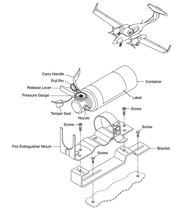
Figure 1B: The Fire Extinguisher Installation of the Fire Extinguisher Amerex 337TS
