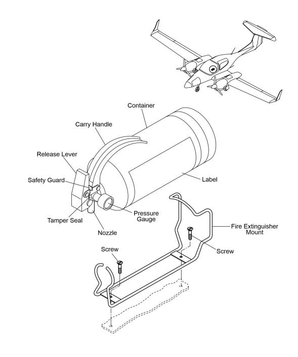
Figure 1: The Fire Extinguisher Installation of the Fire Extinguisher AIR TOTAL HAL 1
