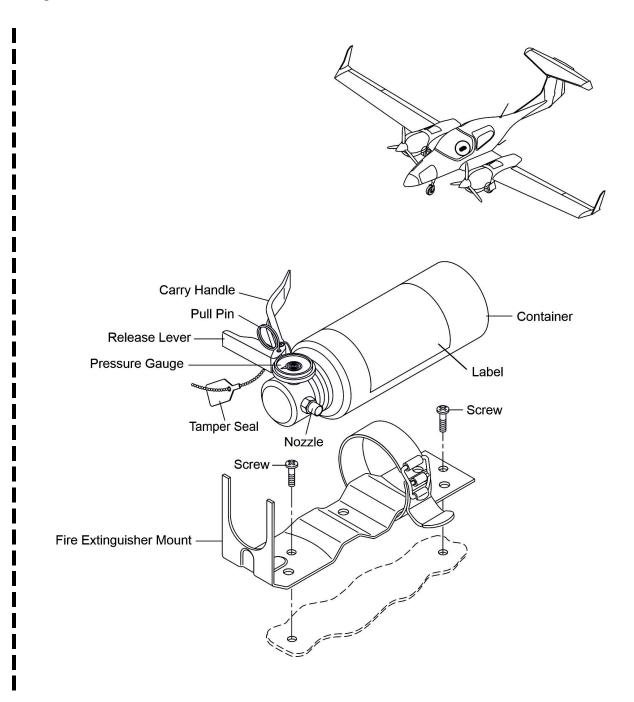
Figure 1A: The Fire Extinguisher Installation of the Fire Extinguisher Amerex A620T
