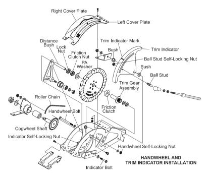
Figure 1: Elevator Trim Mechanism in the Cockpit
