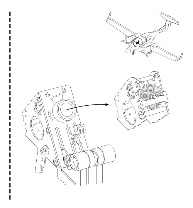
Figure 3: Adjust the Rudder Trim Tab Indication System
