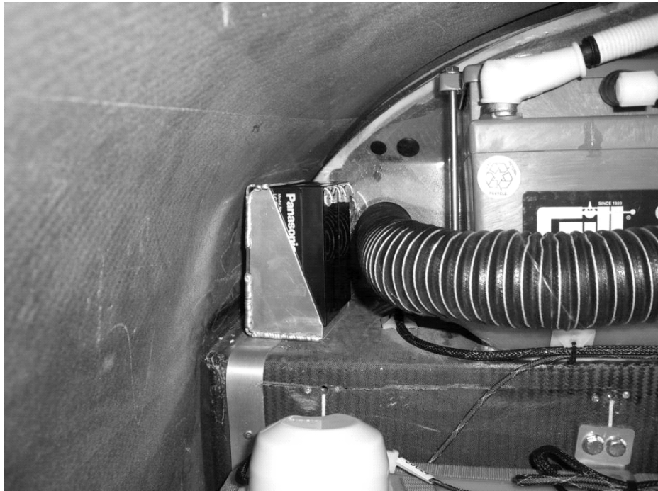
Figure 3: ECU Backup Battery Installation, RH Side (MÄM 42-240 installed)
