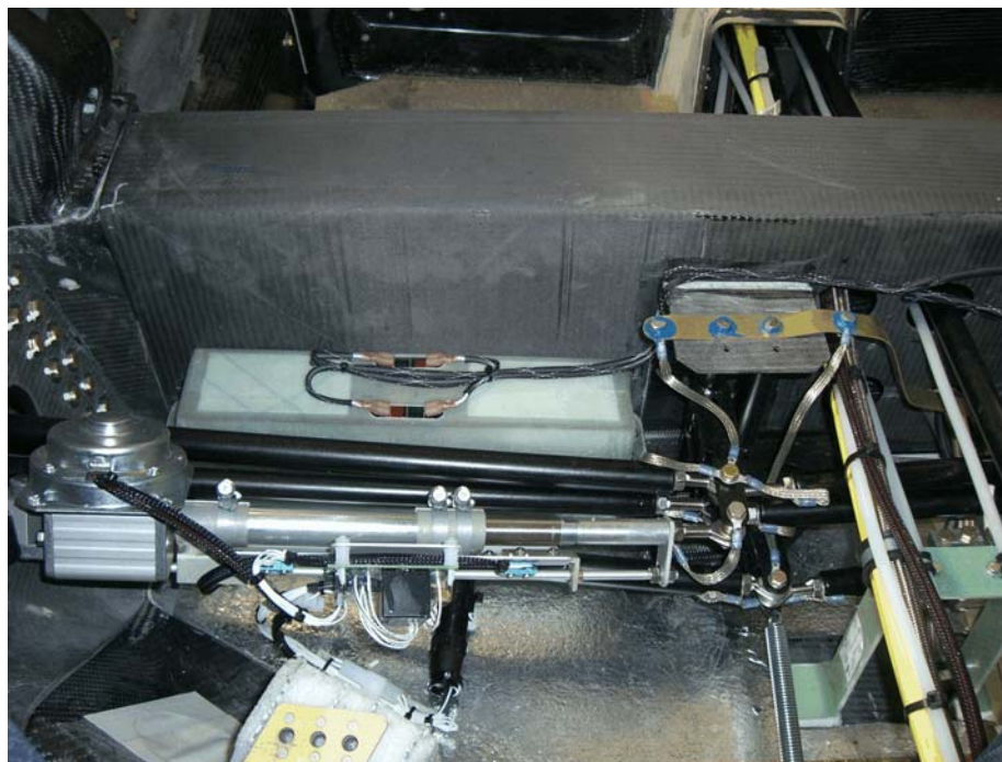
Figure 6: ECU Backup Battery Installation, LH Side (OAM 42-129 installed)
