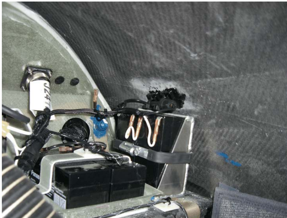
Figure 4: ECU Backup Battery Installation, LH Side (MÄM 42-240 installed)
