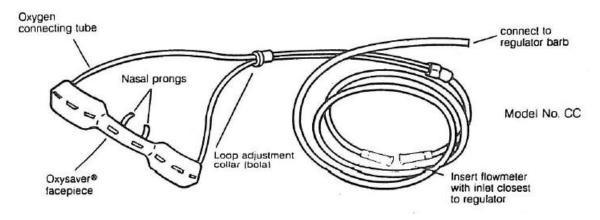
1. Slide the loop adjustment collar (bola) down to enlarge the size of the loop:
