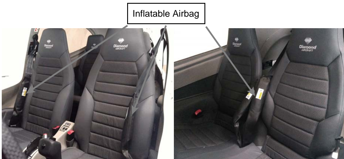
Figure 1 (left): inflatable airbag on lapbelt portion of the three-point restraint (front)
