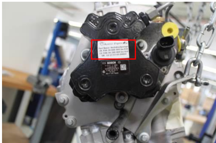
Figure 4 – HPP p/n and s/n location
