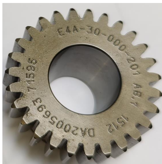
Figure 2 – Driving gear acceptable condition
