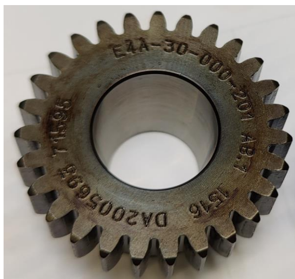
Figure 1 – Driving gear not acceptable condition
