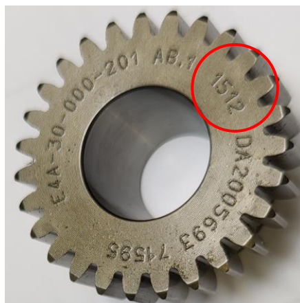
Figure 5 – Gear s/n location
