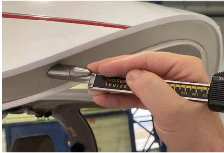
Rear Latching Bolt
