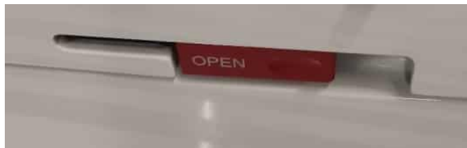
Example: Recessed Passenger Door Handle
