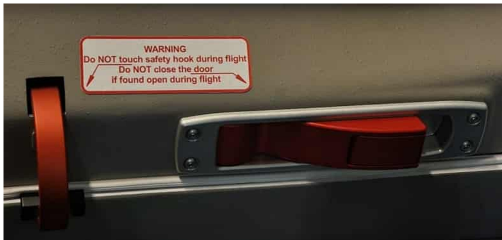
New latching mechanism – MÄM 42-097 installed (refer to step 15)
