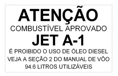
(b) In Addition Next to Each of the Two Auxiliary Fuel Filler Necks (If Installed):
