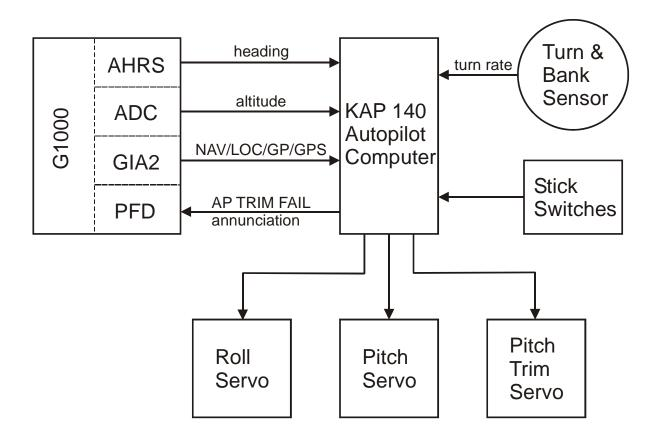
The autopilot computer controls 3 servos: the roll servo, the pitch servo, and the pitch trim servo. It receives information from the G1000, a turn and bank sensor and the stick switches, as shown on the above schematic. The turn and bank sensor for the KAP 140 autopilot is installed behind the MFD and is invisible to the crew. The AP TRIM FAIL annunciation appears on the G1000 PFD. All other autopilot-related annunciations appear on the autopilot computer itself.
