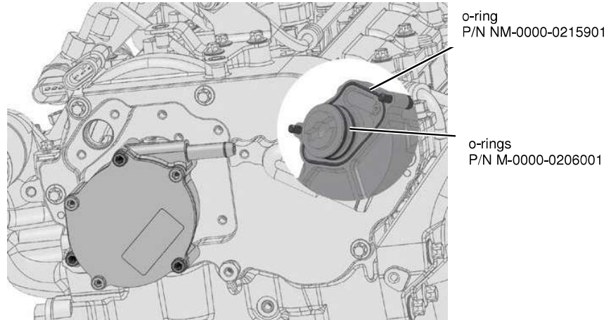
Figure 8 installation vacuum pump
