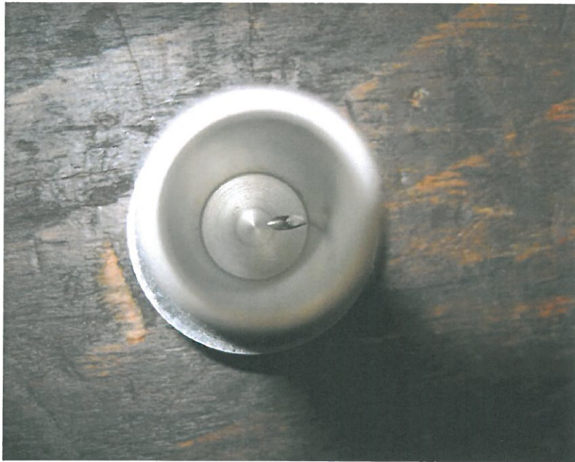
Figure 3 – Chip inside of the oil filler plug
