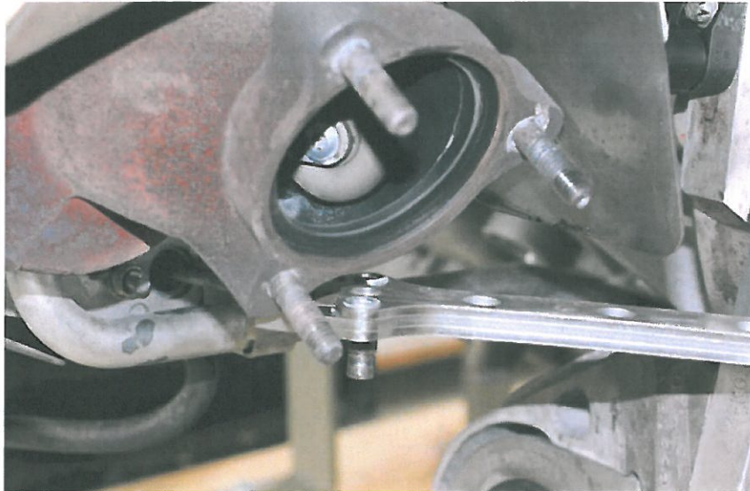
Fig. 2 Hold the waste gate lever steady
