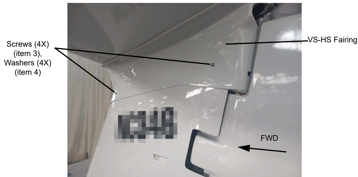
Figure 4. VS-HS fairing installation.
