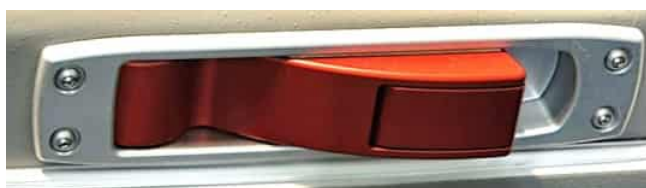
Figure 9. New door latching mechanism (MÄM 40-139 Installed)
