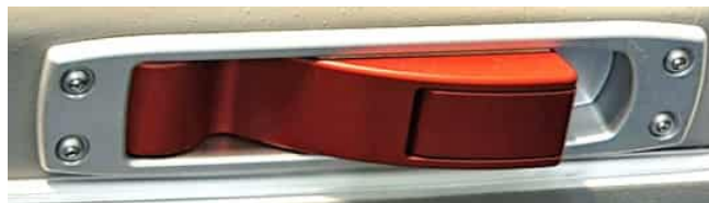
Figure 9. New door latching mechanism (MÄM 40-139 Installed)
