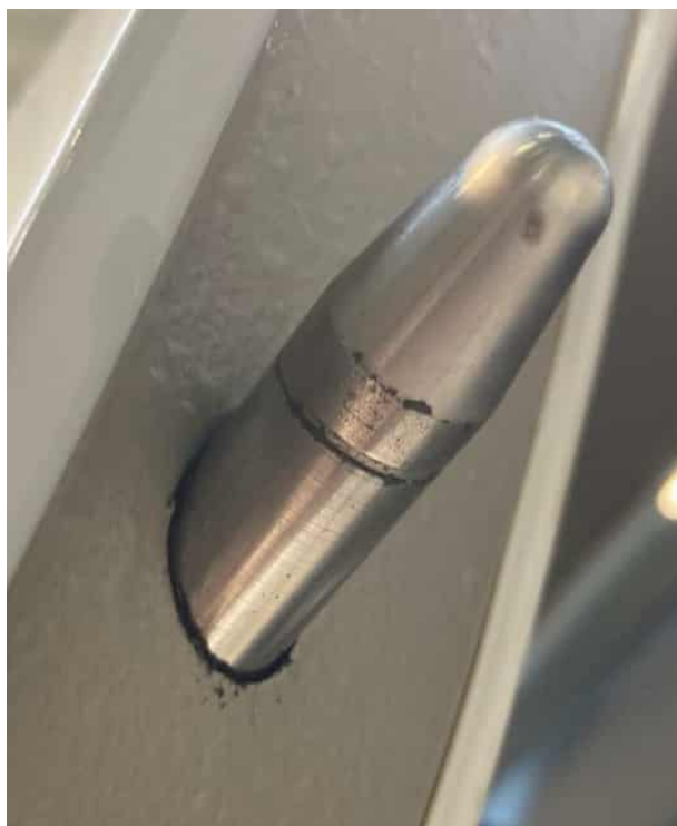
Figure 14. Example of serviceable latching bolt
