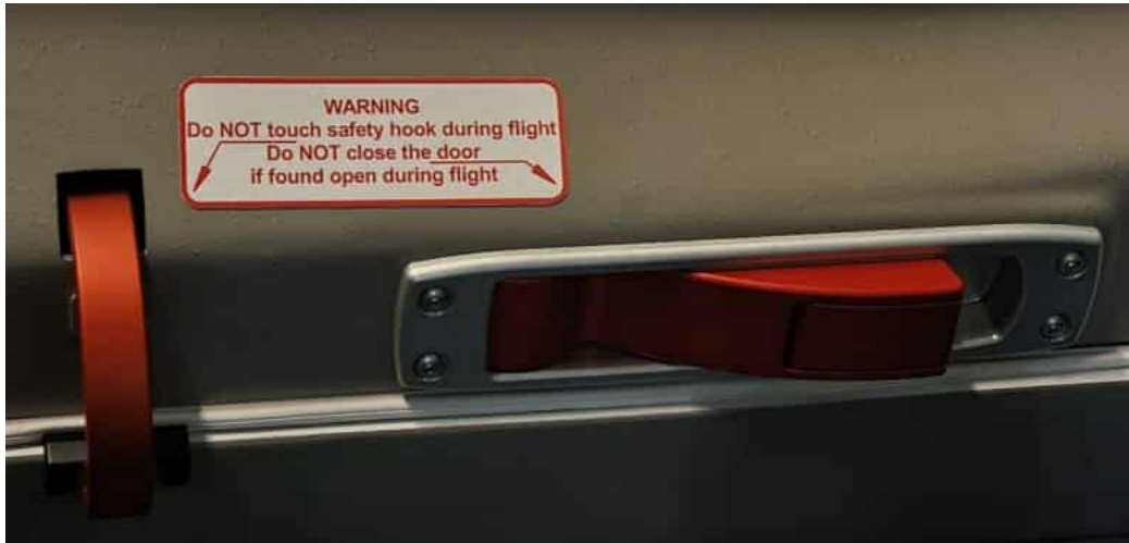
Figure 25. New latching mechanism (MÄM 40-139 installed)
