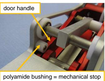
Note: The mechanical stop of the red aluminum door handle must not be defined by the internal stop of the compression gas spring.
