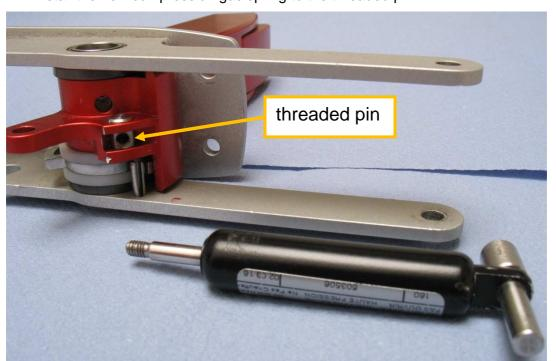
Note: Secure the thread of the compression gas spring with Loctite 243 when installing the new compression gas spring to the threaded pin.
