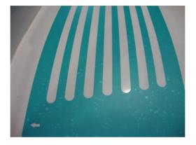
Prepare the surface in the cutouts of the Safety Walk masking foil by carefully roughening the paint with sandpaper (grit 320). Prepare the ends of strips cut out with red Scotch-Brite.
