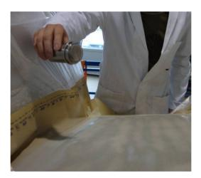
Apply a second layer of lacquer P/N 22101980. Make sure the whole substrate is evenly covered with a sufficient amount of paint.
