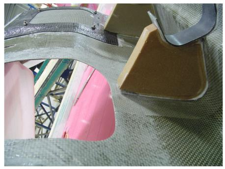
9 position frame kit concisely at the cutout edge, check for regular gap between cut out hole and access cover.
