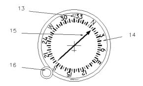
ANT/ADF MODE ANNUNCIATOR - Antenna (ANT) is selected by the 'out' position of the ADF button. This mode improves the audio reception and is usually used for station identification.
