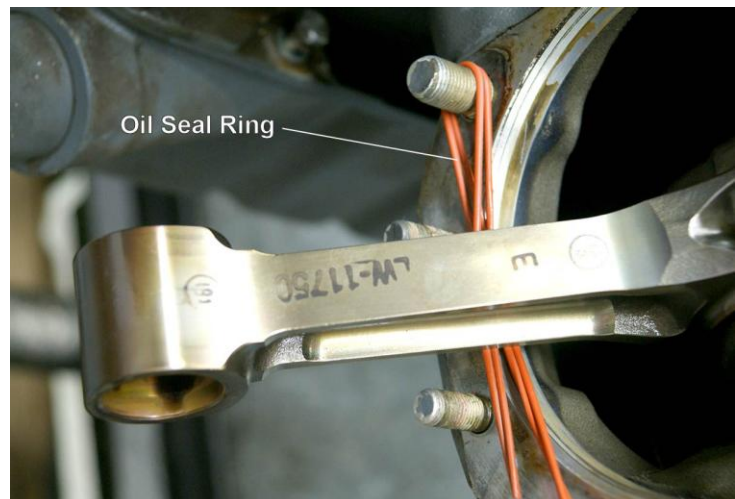
Figure 2 Oil Seal Ring Installed on the Crankcase Studs
