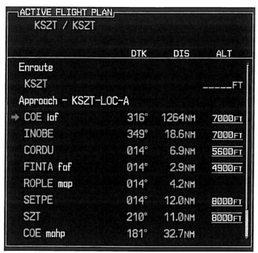
Example V7.00 and later flight plan showing reference altitude for COE iaf.
